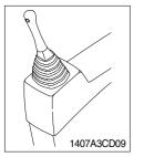
(1) This joystick is used to control the swing and the arm.
