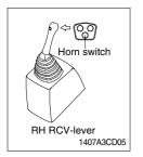
(1) This switch is at the top of right side control lever. On pressing, the horn sounds.
